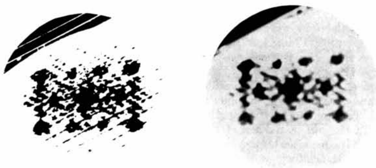
Fig. 4. Photograph of 3-D weighted reciprocal lattice (a) in focus, (b) slightly out-of-focus showing peaks due to anthracene nucleus.
